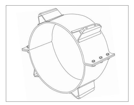
Often it is not possible to lay pipes in open ditches. For example, for rail or road crossings it is first necessary to drive casings underground. By using PSI steel insulators or roller rings, the carrier pipe can be inserted into the casing sleeve safely and efficient.
